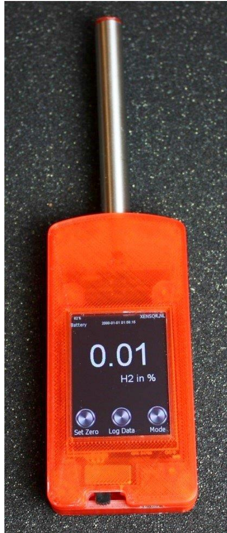
XEN-5320-HAND handheld sensor (210 x 54 x 19 mm)
